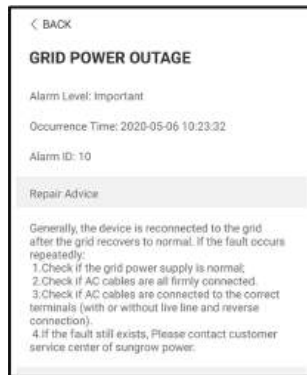
figure 7-9 Detailed Fault Alarm Information
